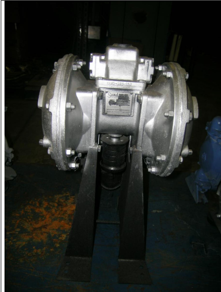
1) Pic no 109& 108 1EA WARREN RUPP 2" "SandPiper" air diaphragm pump w/Air Regulator, water trap & oiler. MOD SB2-A Type DB-1-CI. Cast Iron. 2" quick connect inlet/ outlet. Ser 280795
