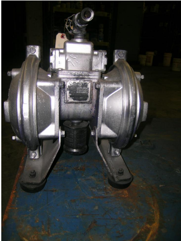
2) Pic no 110 18 EA WARREN RUPP 1 ½” “SandPiper” air diaphragm pump Ser 308313 MOD SB 1 ½ -A Type SB 4-CI Cast Iron 1 ½” quick connect inlet/outlet
