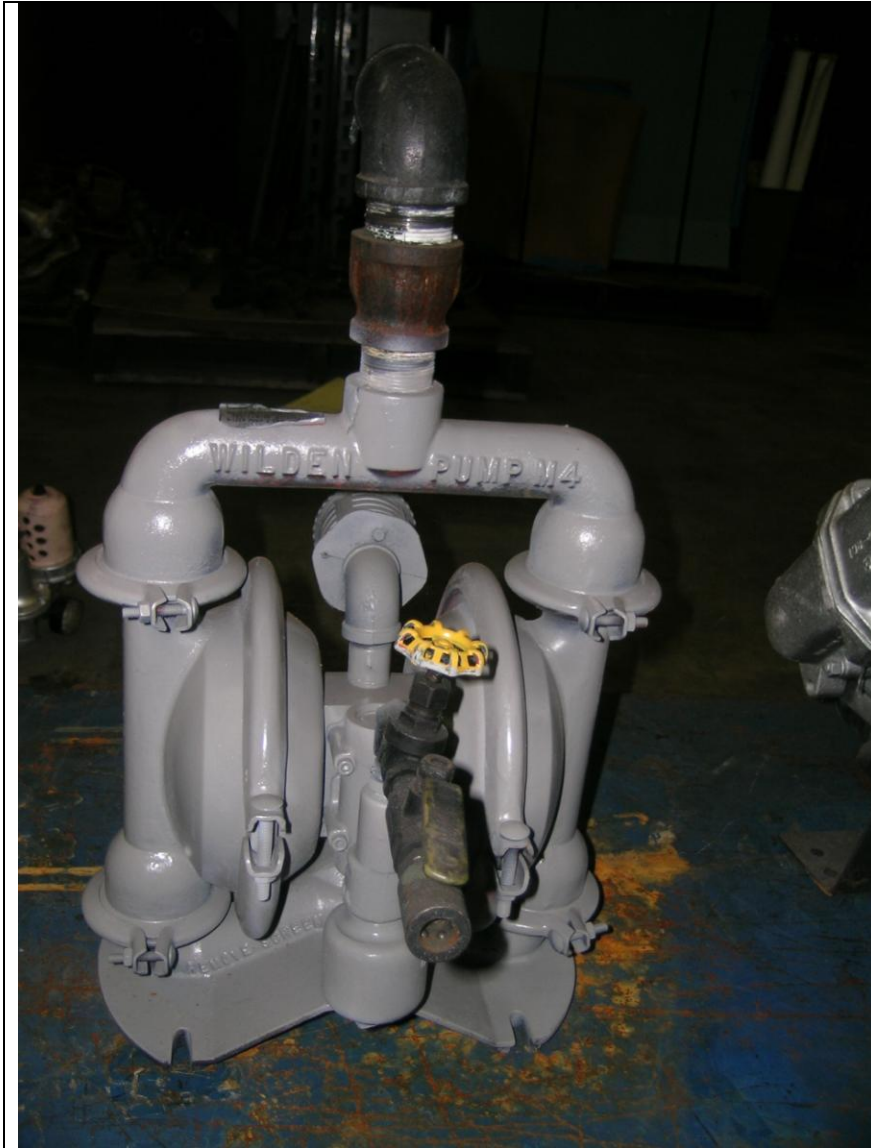
3) Pic no 111 2 EA WILDEN M-4 1 1/2" air diaphragm pump MOD M-4-WO-NE-NE-NE ser 207608 w/ air regulator, water trap & oiler 1 1/2" inlet/outlet
